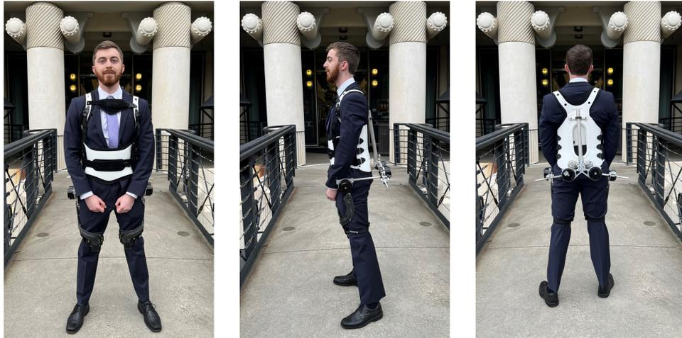
Figure 3.1: Assembled hip exoskeleton without mechatronics. Front (left), side (middle), and back (right) views of the exoskeleton.
