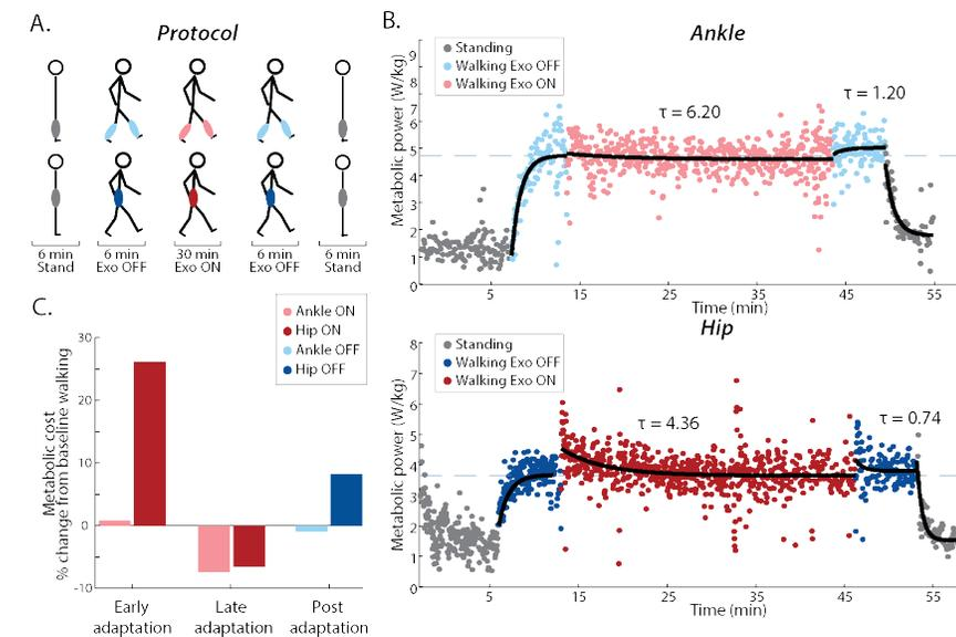
**Figure 1:** (A) Trial structure for an ankle (top) and hip (bottom) exoskeleton. (B) Breath by breath metabolic power during each adaptation trial.  $\tau$  (in minutes) is the time constant of the adaptation and de-adaptation exponential fit. (C) Percent change of mean metabolic cost from steady state walking during early adaptation, late adaptation, and post-adaptation.
