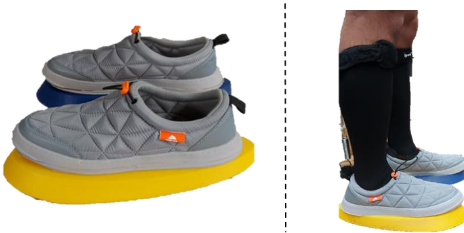
Figure 32 – Final Prototype of the ‘shoe’ portion of the exoskeleton device (left) and the entire system (right). Pinch closures were used for easy slip on and removal.
