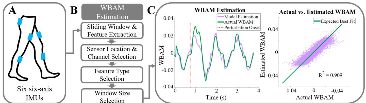
**Figure 1:** (A) We placed IMUs(blue) on the subject's lower limbs. (B) The optimization methods are demonstrated in a flow chart. (C) A time series graph of Actual and Estimated WBAM with an indicated perturbation onset is shown on the left. The correlation graph of Actual and Estimated WBAM is shown on the right where the expected best fit line is plotted in green.
