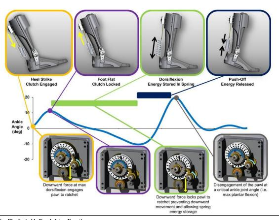
Figure 7. Passive Elastic Ankle Exoskeleton Function
