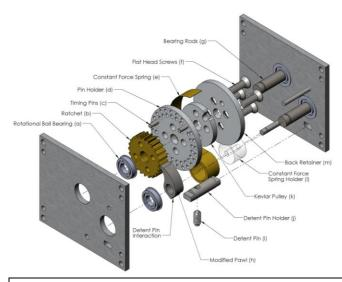
Figure 6. Exploded View of 'Smart-Clutch' Components
