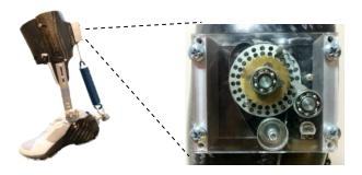
Figure 5. 'Smart-Clutch' for Controlled Energy Storage and Release Prototype clutch with plexi-glass cover (right) and exoskeleton with the clutch coupled to a series spring providing parallel ankle stiffness (left).
