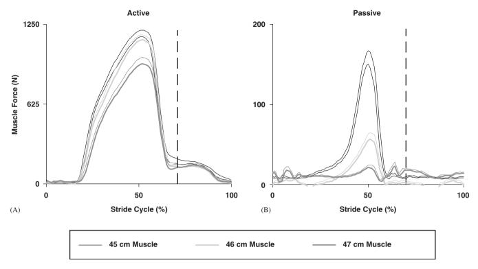
Fig. 6. Maximal muscle length vs. force. Mean + standard deviation of artificial muscle force data from one subject walking at 1.0 m/s during the (A) single active and (B) single passive conditions. Conditions were repeated three times with three different artificial pneumatic muscles fit in the orthosis. Each muscle had a different maximal length (45, 46, 47 cm).
