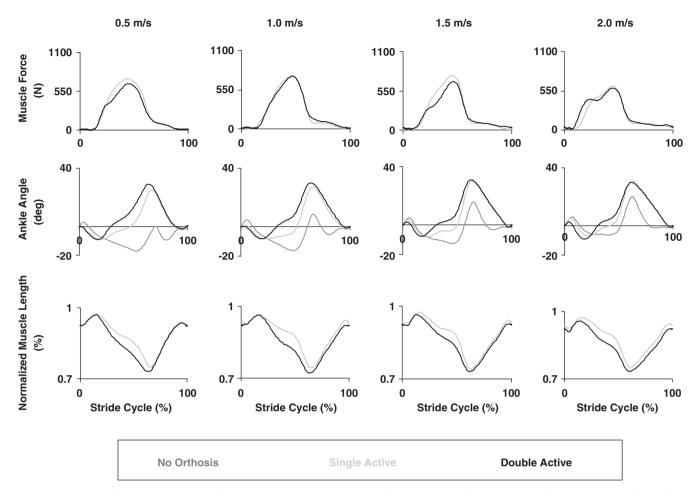
Fig. 5. Mean muscle force, muscle length and ankle angle. Mean artificial muscle force, muscle length and ankle angle from the three subjects at four different speeds during the no orthosis, single active and double active conditions. Data are normalized from left heel strike to left heel strike. Ankle plantar flexion is positive. Zero is neutral ankle angle. 1.0 is maximal artificial muscle length.
